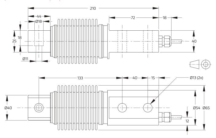
Mounting bolts M12 8.8; torque 90 Nm. Torque value assumes oiled threads.
