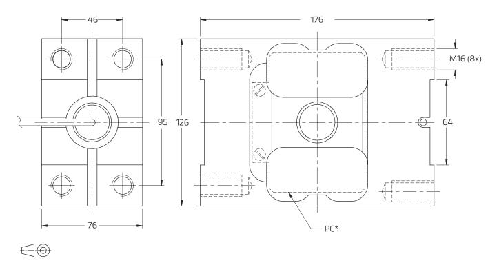
Mounting bolts M16 8.8; torque 200 Nm. Torque value assumes oiled threads. PC\* - Protective cover available on request. 6mm thick, two sides.
